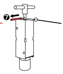
Pull up the firing pin until you can see the hole for inserting the safety device.
